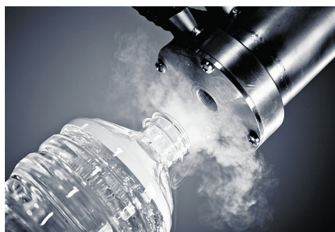
Liquih nitrogen injection into PET on the bottling line with the speed up to 45 000 doses per hour
