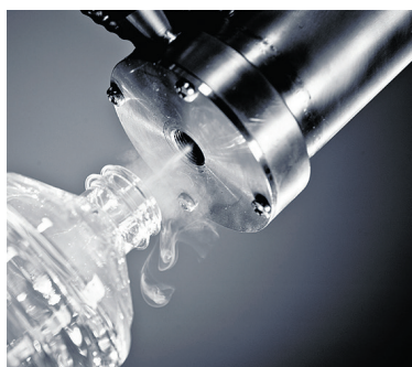
Liquih nitrogen injection into PET on the bottling line with the speed up to 45 000 doses per hour
